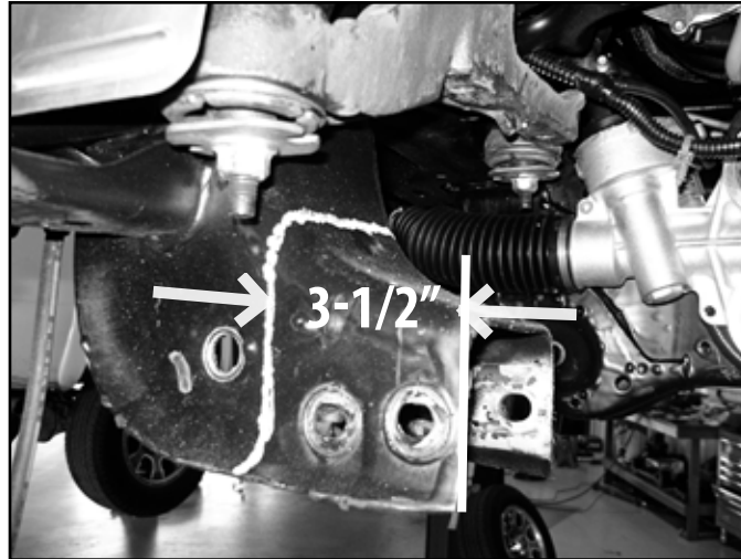
FIGURE 14 - SHOWN WITH DIFFERENTIAL REMOVED FOR CLARITY
