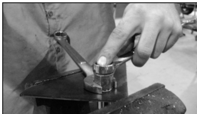
FIGURE 2 - 1/2" RIVET NUT SHOWN
