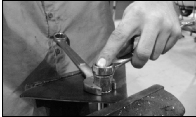
FIGURE 2 - 1/2" RIVET NUT SHOWN
