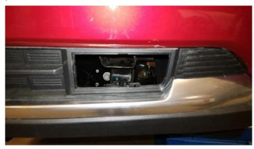
4. Use the Driver Tow Hook Cover as a template to cut the passenger side. Center and mark area to cut.
